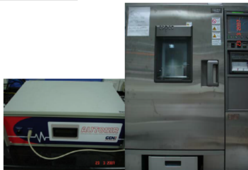
Fig3.Auto-SIR connected with ESPEC Chamber
